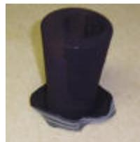
After the panty hose was over the glass I poured activated carbon into the panty hose and glass, packing it with my finger until it was roughly the size of a tennis ball. I then pulled the panty hose up out of the glass and gave it a good shake to make sure the carbon was
